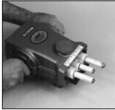
Proper Alignment of Ceramic Plungers for reassembly
